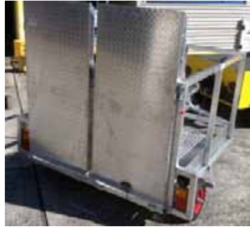
Conditional registration kit including taillights, brake lights, blinkers & number plate light.
