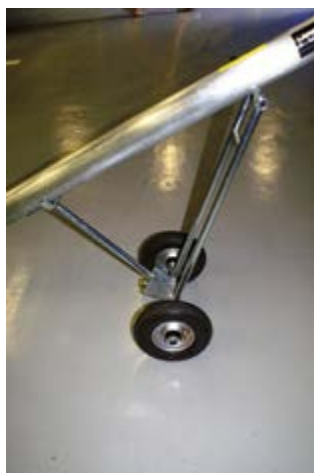
Aux trolley in position
